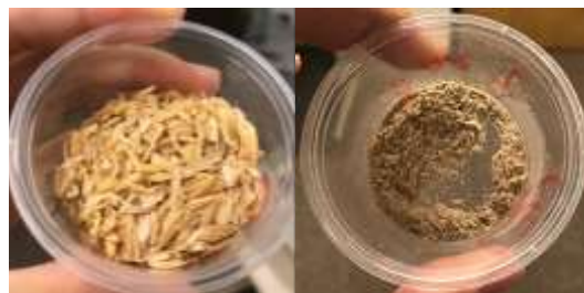
Figure 3: Rice hulls before and after high-energy
