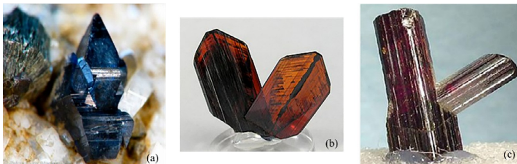
Fig. 1 Crystal forms of \text{TiO}_2 as found in nature (A) Anatase, (B) Brookite, and (C) Rutile.
