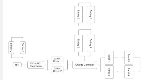
With electrical focus on power, energy is stored in batteries and properly utilized to power and charge all components in the system, such as drivers and step downs.
