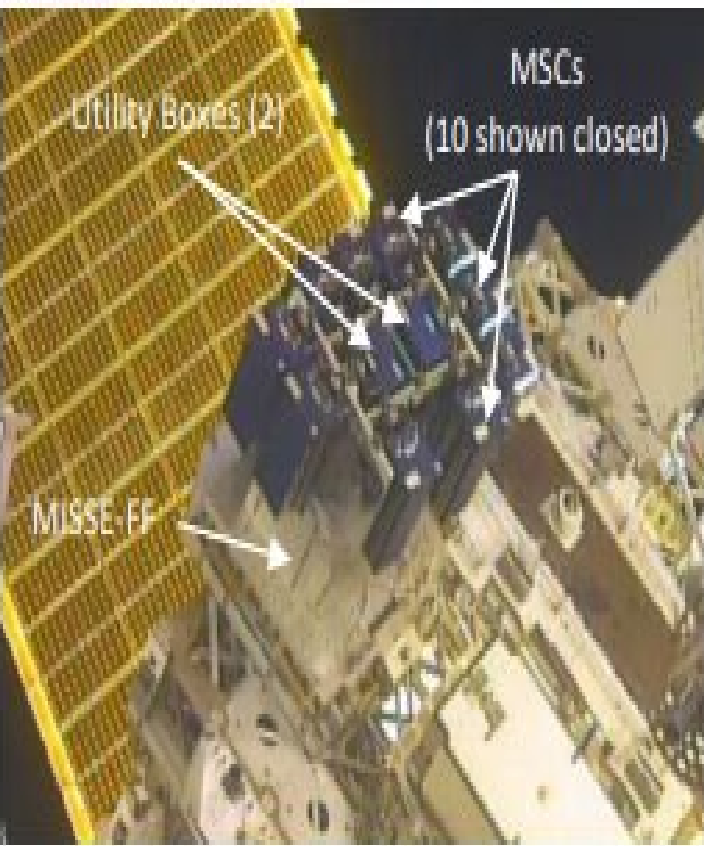
Figure 1a: MISSE On Orbit. The flight facility structure (white) supports two utility boxes (blue in middle) and up to 12 interchangeable MSCs (blue, sides, shown closed).
