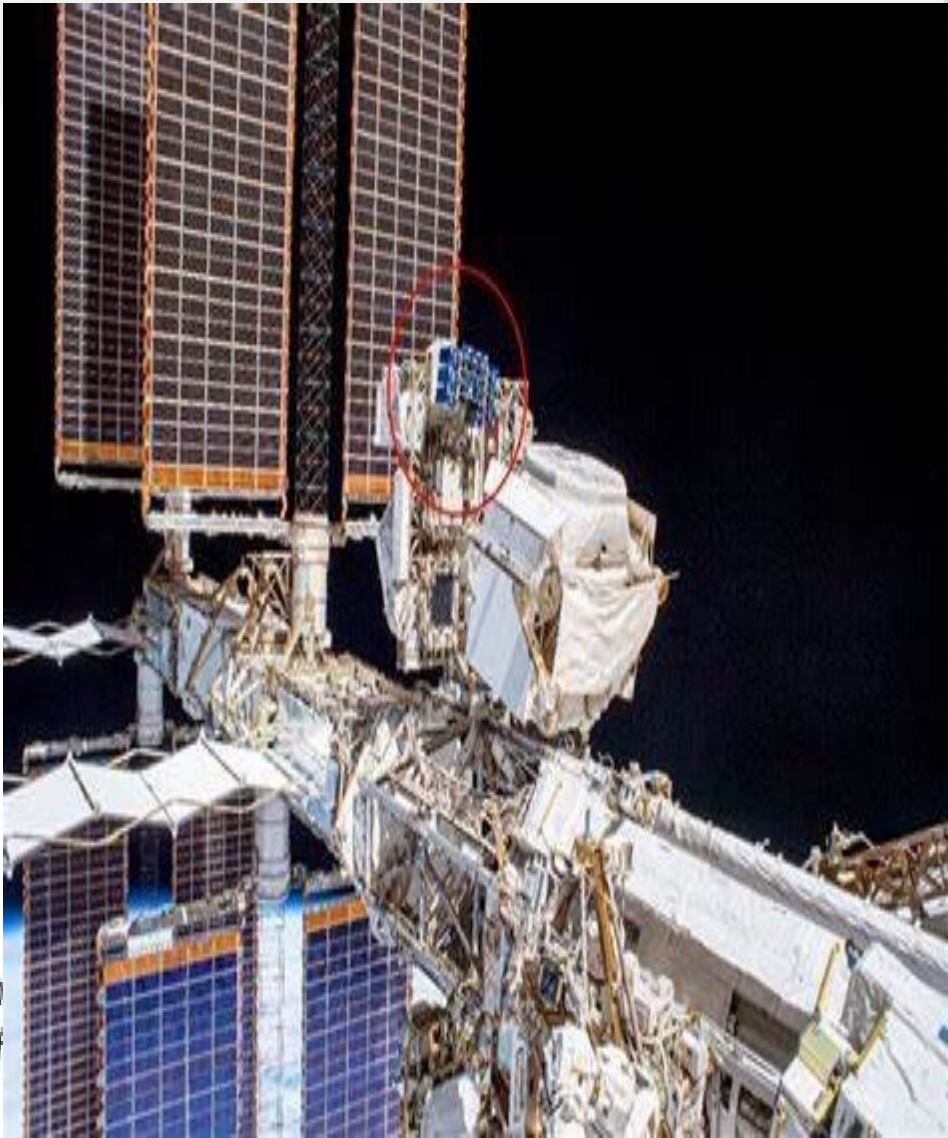
Figure 1b: MISSE On Orbit. View of nadir face (right; on nadir MSC slot is unoccupied) and ram face (left side of image). All MSCs are opened.
