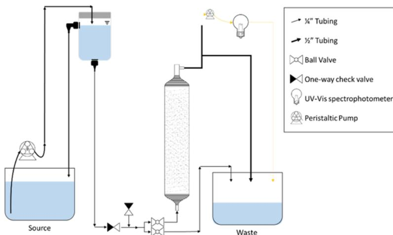
**Figure 1: Experimental column setup**
