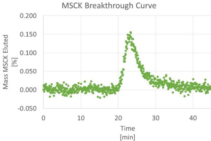
**Figure 2: Breakthrough curve for MCKS in sand**
