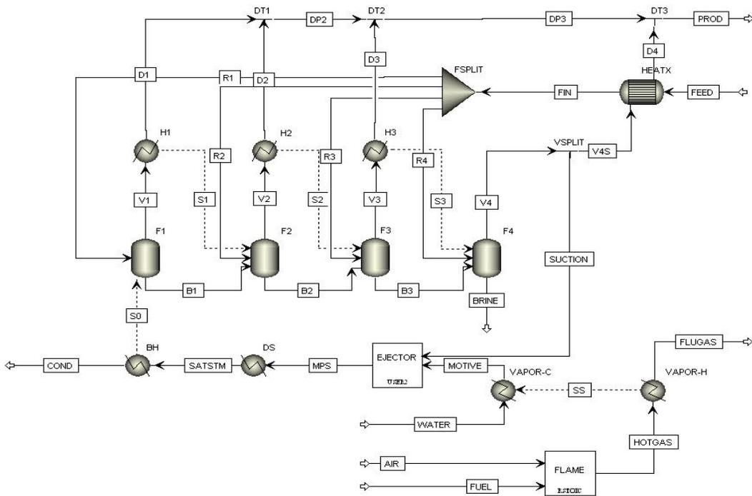
Figure 3. MED desalination process
