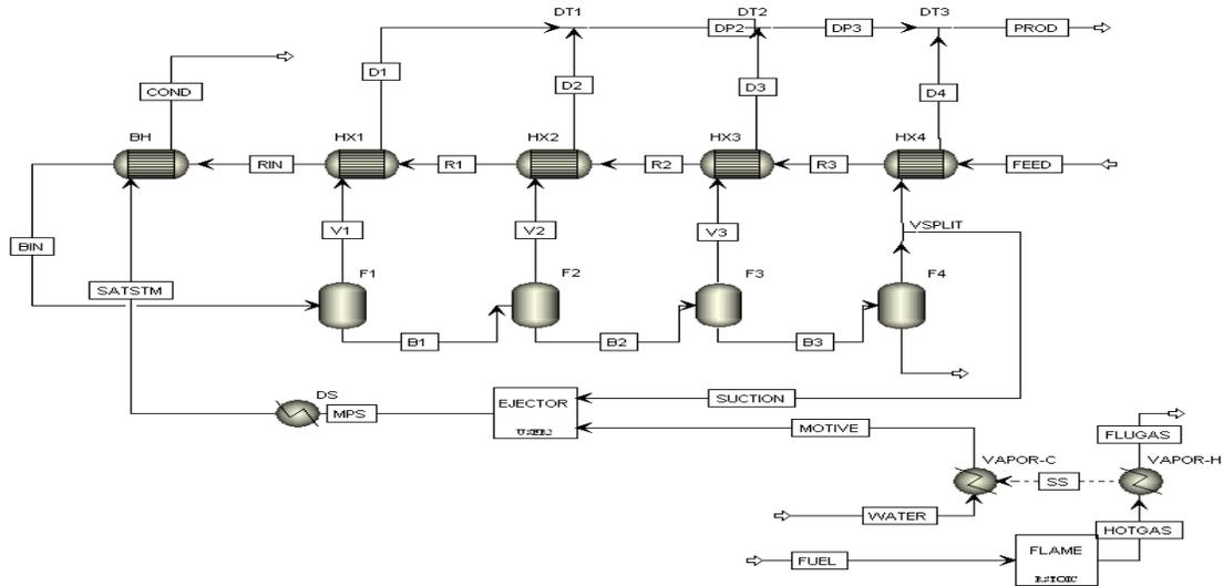
Figure 2. MSF desalination process
