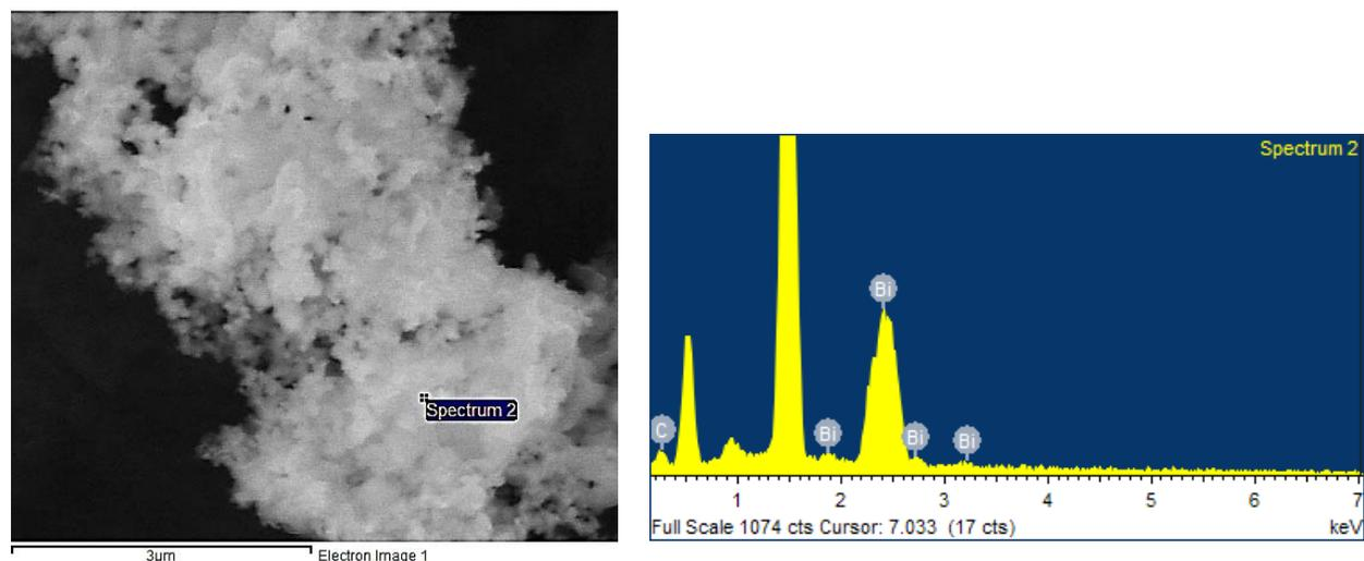
Figure 3. Lipophilic bismuth nanoparticles visualized by scanning electron microscopy. The dominant population of spherical shaped nanoparticles (<100 nm), showed the nanoparticle clusters interspersed among the lesser electron dense material is shown in the TEM images (left). The spectrum of elements in the sample observed by SEM is shown on the right hand side.
