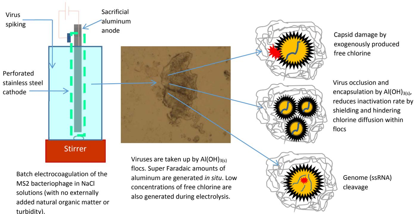
Figure 1. Schematic representation of virus coagulation by electrocoagulation.
