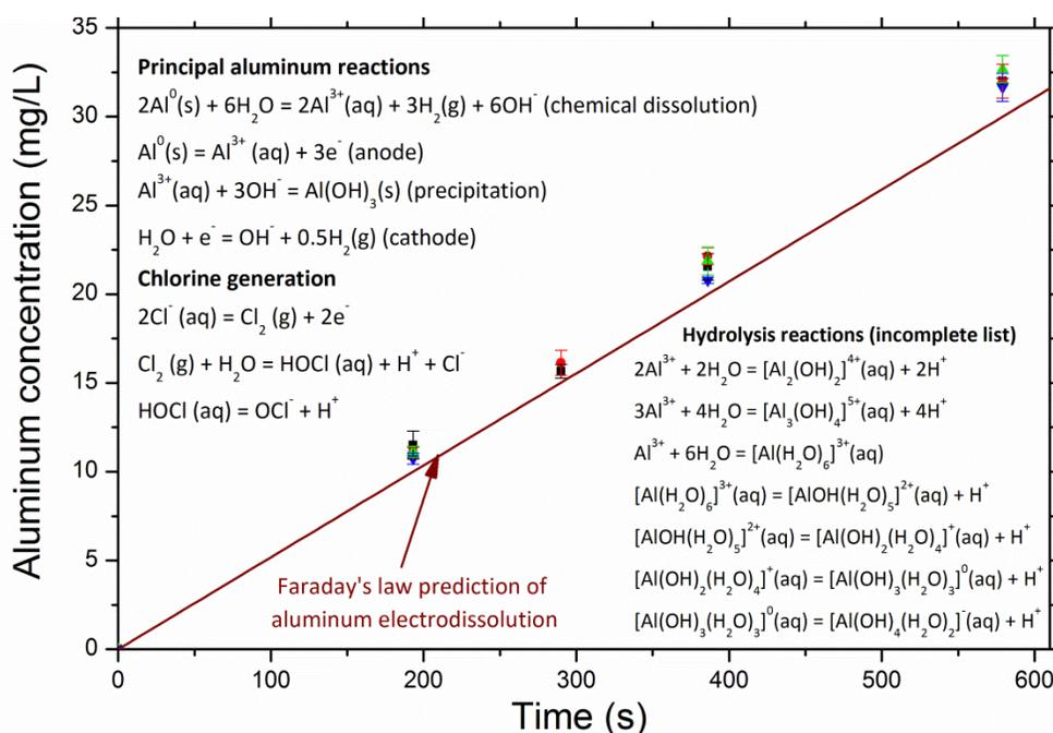
Figure 2. Aluminum electrochemical generation was augmented by chemical dissolution to release more coagulant than predicted by Faraday's law (solid brown line). Expected electrochemical and hydrolysis reactions are also shown. Note that free chlorine is predicted to be generated via oxidation of dissolved chloride ions.
