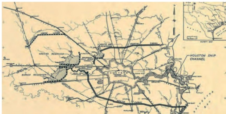
Figure 5: Original 1940 Flood Control Plan for Houston, showing Addicks and Barker Reservoirs to the west, the Cypress Creek levee to the west-northwest, White Oak Reservoir to the northwest, and North and South Canals circling the city and emptying into Galveston Bay to the east. (Source: USACE, 1940).
